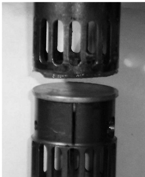
Figure 9. Photos of unloading of the PI sample after a step experiment, without (left) and with (right) having initially imposed a waiting time (5 h).
