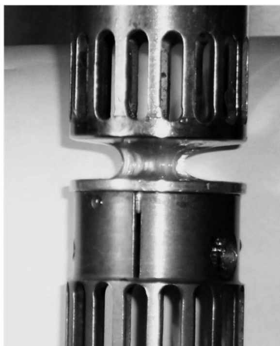
Figure 9. Photos of unloading of the PI sample after a step experiment, without (left) and with (right) having initially imposed a waiting time (5 h).
